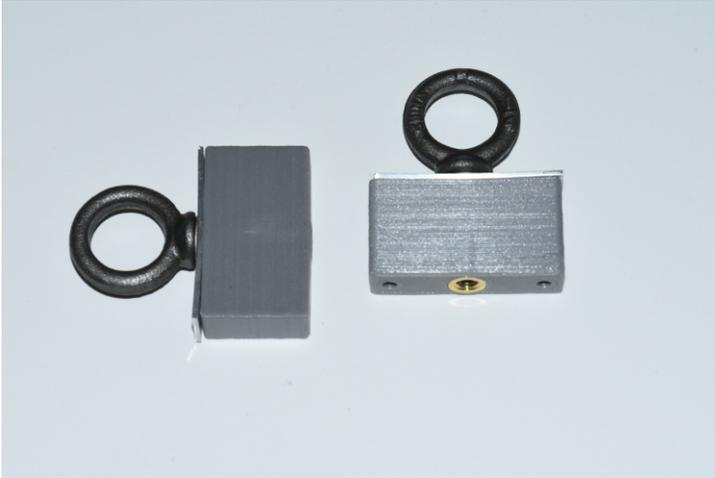
Note: eye bolt has been installed with medium thread locker compound. If the assembly is taken apart, it is important to use thread locker when re-assembling to keep eye bolt in place during flight recovery.
