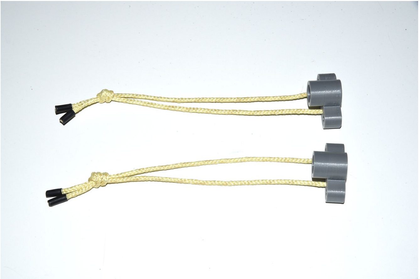
Completed Charge Canister/Shock Cord Tie Assemblies
