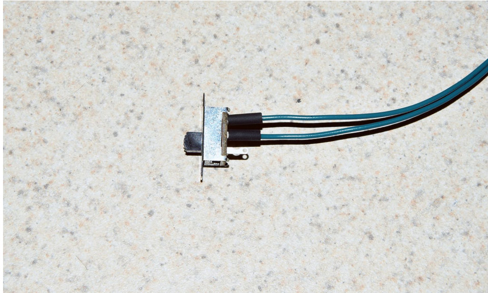
Illustration 7: Slide small section of heatshrink tubing over posts
