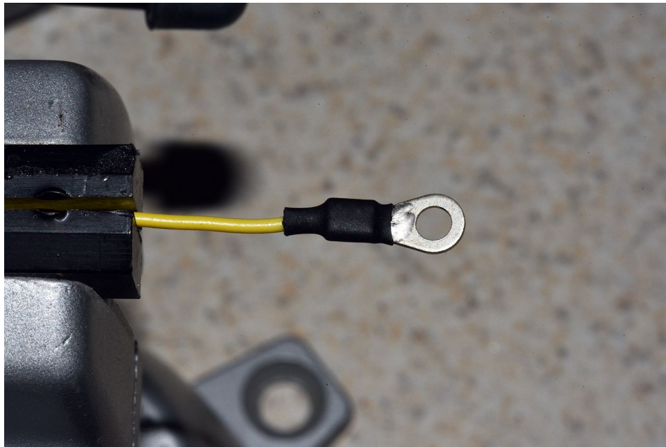
Illustration 5: Slide a section of large heatshrink over lug and shrink tubing
