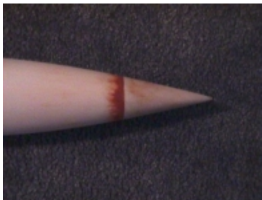
Smoothing the paper extension on the nosecone requires some extra care.
