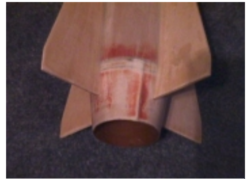
The tailcone detail. As with the nosecone, the tailcone is fabricated from paper.
